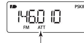
"ATT" appears while the attenuator functions is in use.
